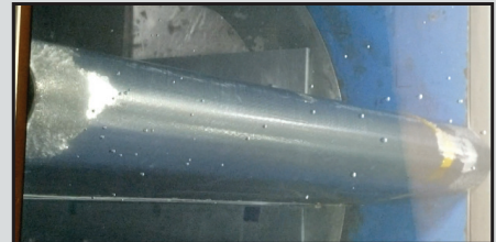
Full ice shed seven seconds after activation
