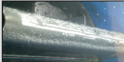
Fully Encapsulated Leading Edge undergoing icing tunnel testing
